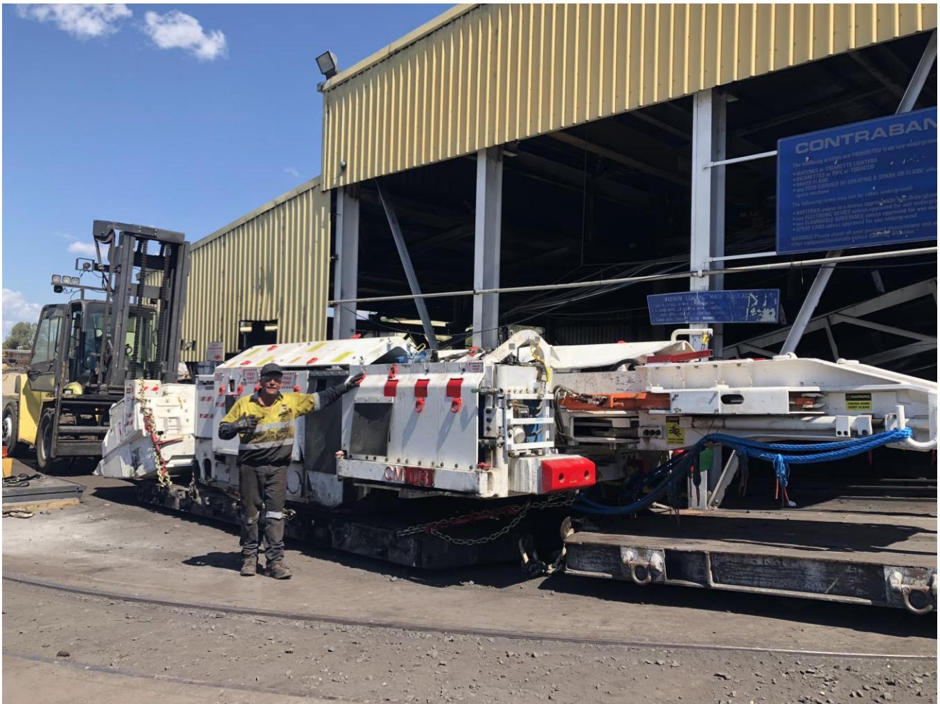
Sumping machine, fully refurbished, and on its way underground in late September.
